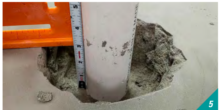
5 The hole is complete when 3 inch depth is achieved at the required hole diameter range, as recommended in step 3.
