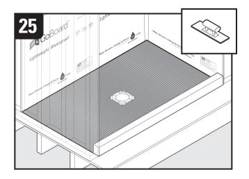
Mix thin set mortar per manufacturers instructions and apply to subfloor using a 3/16'' V-notched trowel. Use a  $1/4'' \times 1/4''$  square notch trowel if additional height is needed or rough subfloor.
