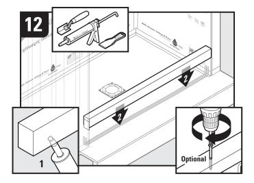
Apply several 1/4" beads on curb (both sections if more than 1 curb required) surfaces in contact with subfloor and walls. Spread excess GoBoard Sealant onto subfloor and curb on shower side. Remove excess sealant on bathroom side of curb.
