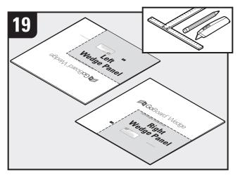
Transfer measurements (for left and right wedge panels) from step 19. Cut wedge panels into rectangles discard remainder. *Note: Thinner side of wedge panel should always face the drain.*
