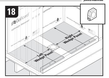
Measure distance between side walls, back wall, curb and clamping collar curb for left and right wedge panels.
