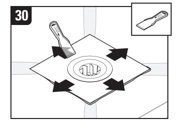
Unfold membrane so it is lying flat over beads of GoBoard Sealant and wedge panels. Using a putty knife, start spreading sealant underneath membrane closest to center of drain moving out. Continue around drain until entire membrane is adhered to wedge panels with sealant.
