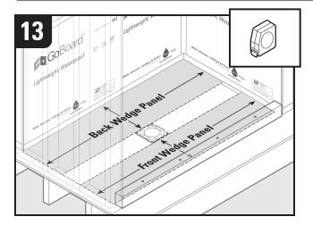
Measure distance between side walls, back wall and clamping collar for back panel and between side walls, curb and clamping collar for front panel. Account for 1/8" gap when measuring and cutting.
