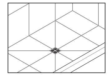
Set remaining tile. After tile installation is complete, grout enclosure and grout or caulk around drain riser and cover. Make sure the drain cover remains removable.
