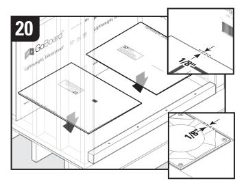
Place wedge panels (left and right) into shower pan area. Note: Thinner side of wedge panel should always face the drain.
