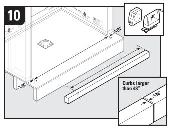
Measure the distance between the left and right walls. Ensure there is a 1/8" gap between curb and side of walls and each curb section if distance is greater than 48". Cut curb section to correct length.
