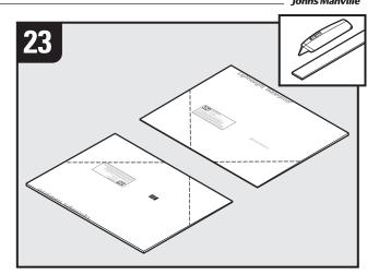
After removing all wedge panels from shower pan, cut along marks to final size. Ensure there is a 1/8" gap at clamping collar, outside walls and between wedge panels.
