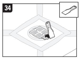
Make all necessary preparations for installing tile. Mix thin set mortar per manufacturers instructions. Using a putty knife, pack thin set mortar underneath drain cover as shown.
