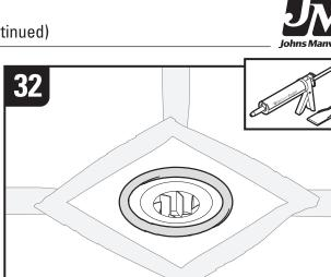
Apply a 1/8" bead of GoBoard Sealant around perimeter of PVC drain flange and spread with a putty knife. Once sealant skins over, begin installing tile.
