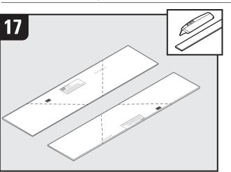
After removing wedge panels from shower pan area, cut along marks on front and rear wedge panels. Dry fit panels to ensure that there is a 1/8" gap at clamping collar, side walls and curb.
