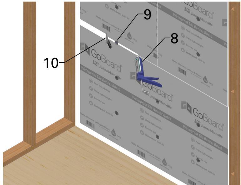
8. Fill 1/8" gaps with GoBoard Sealant or equivalent.
