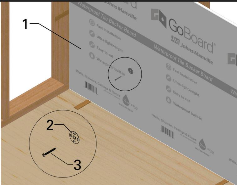
1. Position GoBoard LT. Use shims or spacers to ensure 1/8" gaps.
