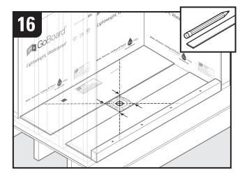
Locate the drain center and mark 45° angles on **left** and **right** wedge panels as shown (use corners of clamping collar as reference points to draw cut lines).
