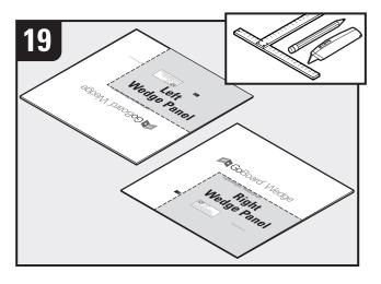
Transfer measurements (for **left** and **right** wedge panels) from step 19. Cut wedge panels into rectangles discard remainder.
