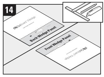
Transfer measurements (for **back** and **front** wedge panels) from step 14. Cut wedge panels into rectangles (discard remainder). **Note:** Thinner side of wedge panel should always face the drain. Use straight edge for cut.
