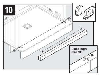
Measure the distance between the left and right walls. Ensure there is a 1/8" gap between curb and side of walls and each curb section if distance is greater than 48". Cut curb section to correct length.
