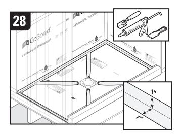
Fill 1/8" gaps, including between clamping collar and wedge panels, with sealant and spread excess sealant with a putty knife at least 1" from either side of 1/8" gaps. For the 90 degree inside corners, use a 90 degree putty knife to ensure the inside corners are completely sealed.
