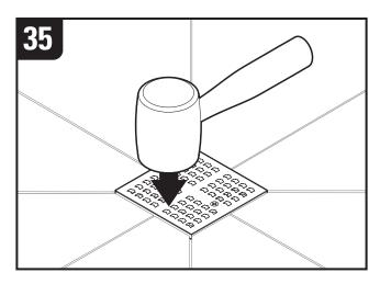
Begin installing tile around drain. Using a rubber mallet, gently level drain cover with surrounding tile if needed.
