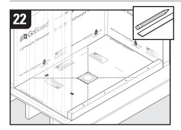
Using **front** and **back** panel edges, mark 45 degree angles on **left** and **right** wedge panels.
