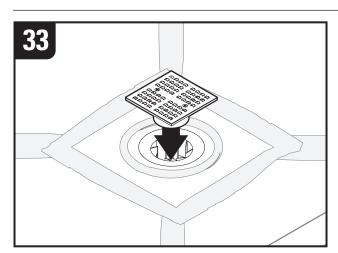
Install the drain cover assembly into the center of the drain. The radial fins are designed to accommodate most 2" drain cover assemblies while allowing for easy removal and repositioning during tiling. The final height of the drain cover needs to match the height of the installed tile.
