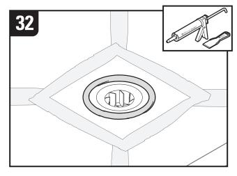
Apply a 1/8" bead of GoBoard Sealant around perimeter of PVC drain flange and spread with a putty knife. Once sealant skins over, begin installing tile.
