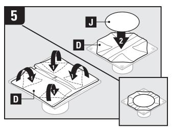
Fold corners of membrane (D) inward so that screw holes are readily accessible. Add tape dot (J).
