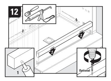
Apply several 1/4" beads on curb (both sections if more than 1 curb required) surfaces in contact with subfloor and walls. Spread excess GoBoard Sealant onto subfloor and curb on shower side. Remove excess sealant on bathroom side of curb.
