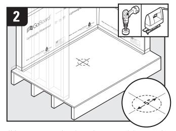
Using measurements from the previous step, mark the center of the drain hole. Cut a 5" diameter hole with jig-saw, hole saw or other means. For remodels, ensure existing drain location fits within the layouts and dimensions outlined on page 10 and 12.
