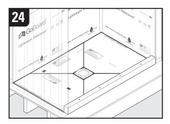
Dry fit all four wedge panels to ensure that there is a 1/8" gap between wedge panels, clamping collar, side walls and curb.
