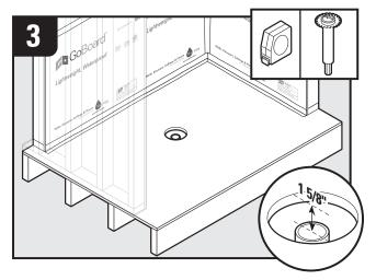
Top of waste pipe **MUST** be at least 1 5/8" below the top of the subfloor. For remodels, cut existing waste pipe as needed with inside pipe cutting tool.
