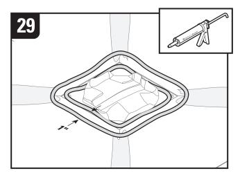
After removing tape dot and folding membrane edges up, Apply a 1/4" bead of GoBoard Sealant on top of clamping collar near folded membrane, fill remaining gaps between clamping collar and wedge panels and apply another 1/4" bead of sealant around the perimeter of the drain base approximately 1" from clamping collar as shown.
