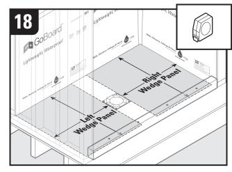
Measure distance between side walls, back wall, curb and clamping collar curb for left and right wedge panels.
