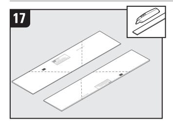
After removing wedge panels from shower pan area, cut along marks on front and rear wedge panels. Dry fit panels to ensure that there is a 1/8" gap at clamping collar, side walls and curb.
