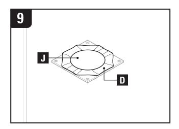
Refold membrane (D) and secure corners with tape dot (J) see steps 5 and 6) so that edge of clamping collar is exposed.
