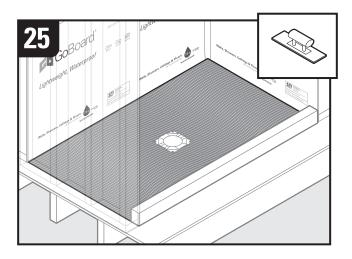
Mix thin set mortar per manufacturers instructions and apply to subfloor using a 3/16" V-notched trowel. Use a 1/4" x 1/4" square notch trowel if additional height is needed or rough subfloor.
