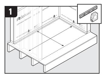
Make sure floor is level (floor **must** be level for proper installation). Find the center of the shower pan area (or as close to center as framing allows). Please review page 10 for possible layouts.
