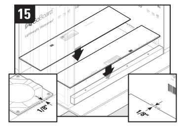
Place wedge panels (**front** and **back**) into shower pan area. Ensure that there is a 1/8" gap at clamping collar and side walls. **Note:** Thinner side of wedge panel should always face the drain.
