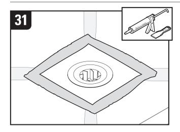
Spread excess GoBoard Sealant around perimeter of membrane as shown in illustration.
