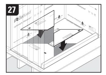
Install **front** and **back** cut wedge panels by pressing firmly into thin set. Ensure that there is a 1/8" gap at clamping collar, side walls, curb and wedge panels.
