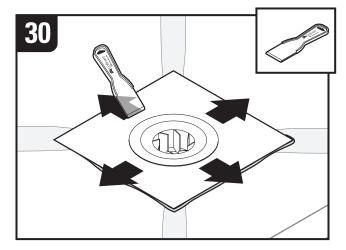
Unfold membrane so it is lying flat over beads of GoBoard Sealant and wedge panels. Using a putty knife, start spreading sealant underneath membrane closest to center of drain moving out. Continue around drain until entire membrane is adhered to wedge panels with sealant.
