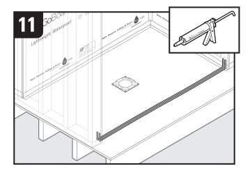
In curb location, apply two 1/4" beads of GoBoard Sealant.
