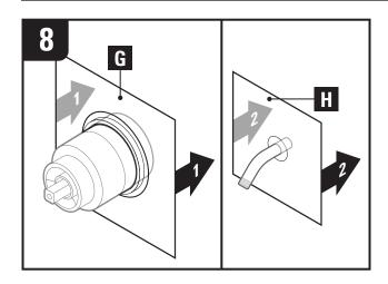
Install valve seal (G) over valve and waterproof pipe seal (H) over shower pipe using GoBoard Sealant.
