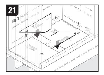
Place cut **front** and **back** wedge panels back in shower pan area on top of uncut **left** and **right** wedge panels.
