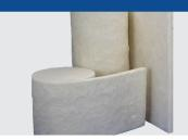
A lightweight insulation made from rotary-process fiberglass. Provides excellent thermal performance for commercial and residential applications operating at hot-face temperatures up to 1000° F. While Spin-Glas WH XG / Range-Glas XG is made with a formaldehyde-free binder, first exposures of the insulation to elevated temperature ( $\geq$  450°F), will result in some formaldehyde emissions.
