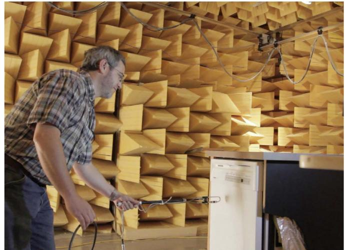
An intensity probe is used for both scanning and point to point mapping of power radiated from a simulated aircraft fuselage. Such techniques measure the attenuation of the overall system as well as the performance of specific elements within the construction.
