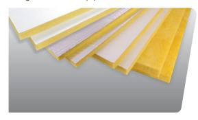
800 Series Spin-Glas® is a fiberglass equipment and external duct insulation offered in a variety of different densities. The board is available plain or with a vapor-retarder FSK, AP, or Ultra (poly-top) facing. The insulation can be readily cut with a knife and secured in place with mechanical fasteners and/or adhesives.
