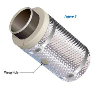
4.4.2.2 Weep holes should range from 1/2" - 1" in diameter.
