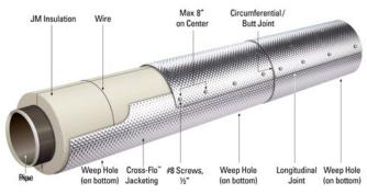
4.5.3.4 Screws shall be installed at a maximum spacing of 3" on center on the longitudinal joint of elbow covers. Refer to Figure 13.
