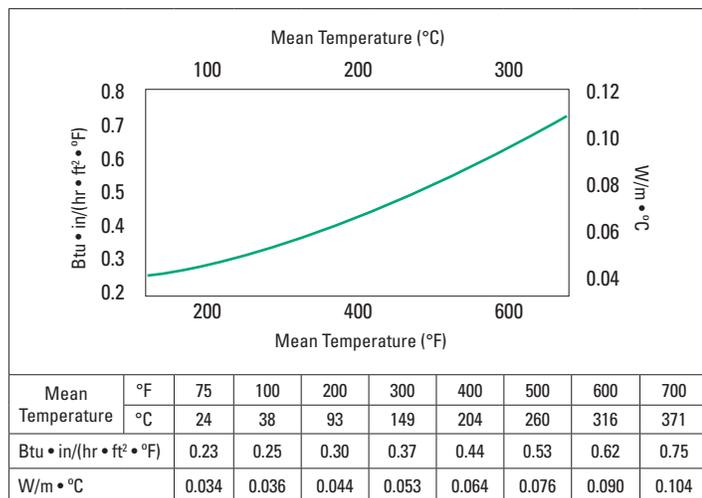
\* MinWool-1200 Field-Formed Pipe Insulation as tested in accordance with ASTM C518.
