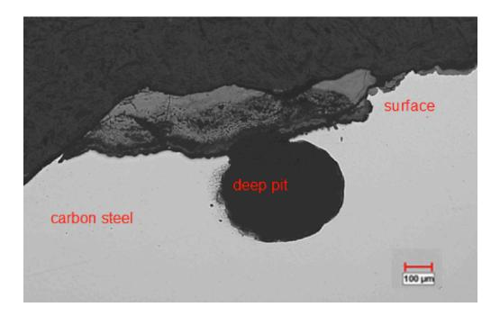
Figure 1: Optical cross-section of a carbon steel surface under the tested silicaaerogel blanket insulation after high-temperature cycling conditions, showing deep, localized pitting. Deep, localized pitting is more concerning than uniform shallow pits.
