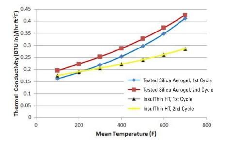
Figure 2: Thermal conductivity values tested via ASTM C335 before (1st cycle) and after (2nd cycle) thermal shift. Note the thermal conductivity values for InsulThin HT do not vary between the 1st and 2nd cycles.
