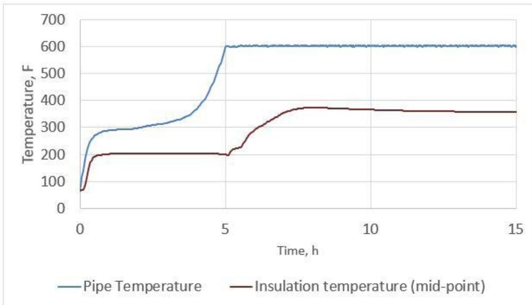
This temperature plateau is the result of the decreased efficiency of the water-logged insulation. The system takes longer to heat up because the insulation is more thermally conductive until it becomes dry enough to operate efficiently. Ultimately, after hours at approximately 200°F, the temperature of the insulation in Configuration C can be seen breaking through the plateau as it expels enough water to become thermally efficient once again.
