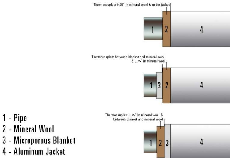
wool binder burnout, and as the outer layer to prevent water ingress in situations when the jacketing may be compromised. The microporous blanket was cut to size to wrap around either the 3” metal pipe when used as the inner layer or at 6” diameter (i.e., 3” pipe plus 1.5” thickness insulation) when used as the outer layer. A single, 10-mm thick layer was used for both configurations.
