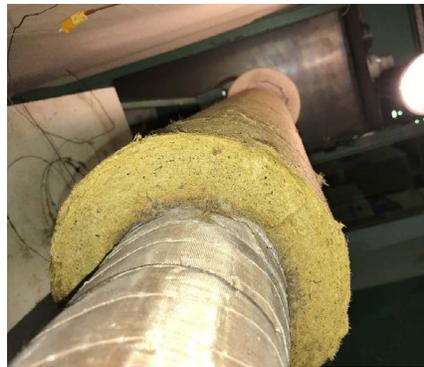
**Figure 4. Configuration C: Binder burnout extends to outer surface of the mineral wool when microporous blanket is used on the outside.**
