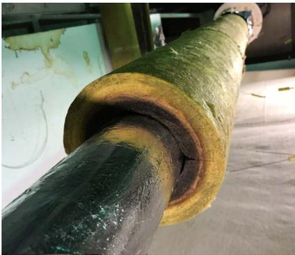
**Figure 3. Configuration B: Binder burnout during conditioning was significantly reduced when the microporous blanket was used as inner layer**
