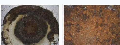
The relative concentration of iron or iron oxide in the samples corresponds to the relative performance of the insulations in the ASTM C1617 corrosion test method.
