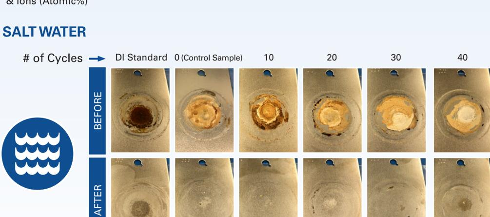
Although the relative amounts of the protective layer deposited by the XOX Corrosion Inhibitor varied somewhat over the course of the testing, they did not diminish over time for either environmental condition. The minor variations we saw in the surface layer composition are caused by variations in the base chemistry of the insulation, and not by the material gaining or losing its corrosion inhibiting properties as a result of wet-dry cycling.
