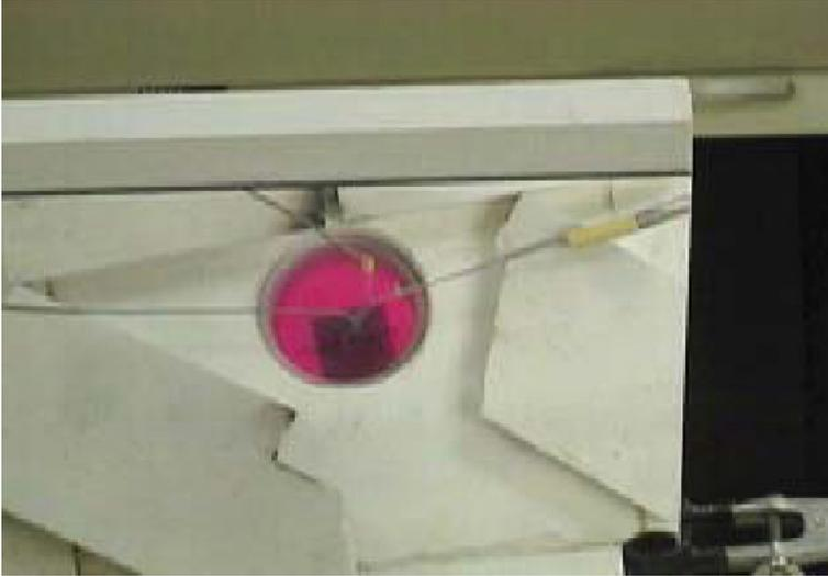
**Figure 1:** A test specimen of calcium silicate 35 seconds after being inserted into the center of an <sup>1</sup>ASTM E136 furnace. Notice that there is no flame visible. Further, the specimen's surface temperature and interior temperature remained close to 1382°F (750°C), the original furnace temperature.
