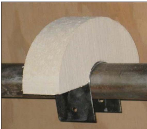
**Figure 2** – Sample of insulation resting on top of steel “U” bend coupons. This is the procedure specified in the ASTM C692 test method.
