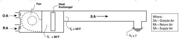
The size of the cooling coil is determined by the volume and condition of the supply air required by the space cooling load. For many reasons, one of which was discussed in the Engineering & Technical Bulletin dealing with condensation control on air conditioning ducts (80-1-ISD), the drop in the air temperature across the cooling coil is limited to  $30^{\circ}F \pm 5^{\circ}F$  for most HVAC systems. The coil sensible cooling capacity is determined by the following equation:
