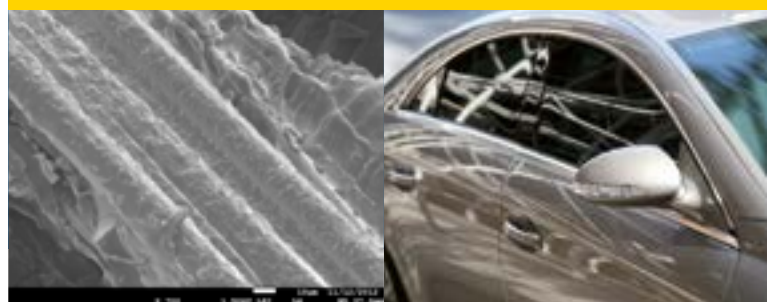
SEM picture indicating excellent matrix-glass bonding in PA6 system
