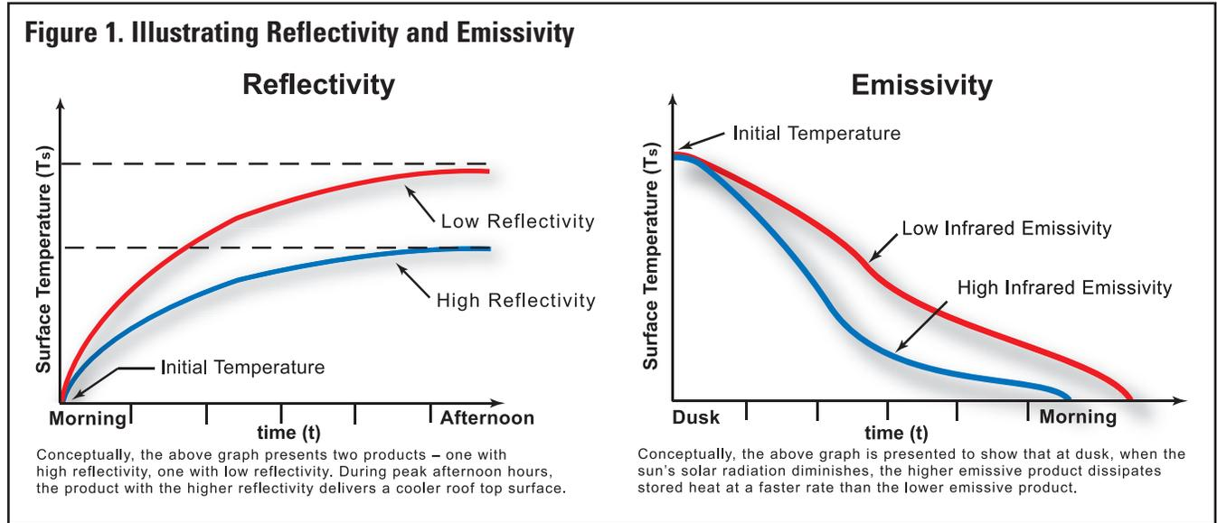
Energy efficient material selection will impact indoor environmental comfort, which results in lower energy consumption and reduced demand during peak periods.
