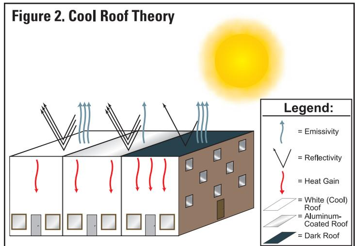
Figure 2 above is presented in a simplified form to illustrate the theory of cool roofs. There are many complex and related variables that must be considered when selecting the correct roofing product for the application.
