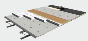
Optional solution where at least one layer of the roofing system above is fastened through to the deck/structure below
