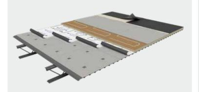
All layers of the roofing system above are adhered
