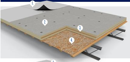
(Adhered, fastened or induction-welded)
