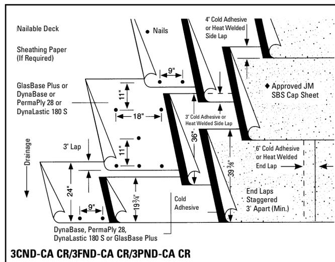
Roll a 19 3/4" (502 mm) wide piece of one of the intermediate felts listed into a full coating of MBR Cold Application Adhesive or MBR Bonding Adhesive. The remaining felts are to be applied full width, in the same manner. End and side laps can be done in one of the following ways:
