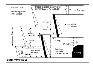
Heat weld a full width piece of one of the cap sheets listed so that it is firmly and uniformly set. Subsequent sheets are to be applied in the same manner, with 4" (102 mm) side and 6" (152 mm) end laps over the preceding sheets. All laps must be rolled with a 3" (76 mm) rounded edge roller. A  $\frac{1}{6}$ " to  $\frac{3}{6}$ " (3 mm to 10 mm) bleedout of APP compound shall be visible at the edge of all seams. All laps must be checked for good adhesion.
