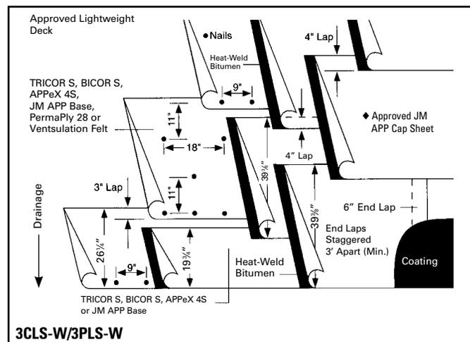
Heat weld a full width piece of one of the cap sheets listed so that it is firmly and uniformly set. Subsequent sheets are to be applied in the same manner, with 4" (102 mm) side and 6" (152 mm) end laps over the preceding sheets. All laps must be rolled with a 3" (76 mm) rounded edge roller. A ⅛" to ⅜" (3 mm to 10 mm) bleedout of APP compound shall be visible at the edge of all seams. All laps must be checked for good adhesion.
