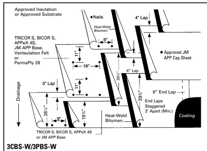
Over the fastened base ply, heat weld a 19¾" (502 mm) piece of one of the intermediate plies listed with 4" (102 mm) side and 6" (152 mm) end laps. The remaining plies are to be applied full width, in the same manner, with 4" (102 mm) side and 6" (152 mm) end laps over the preceding sheet.
