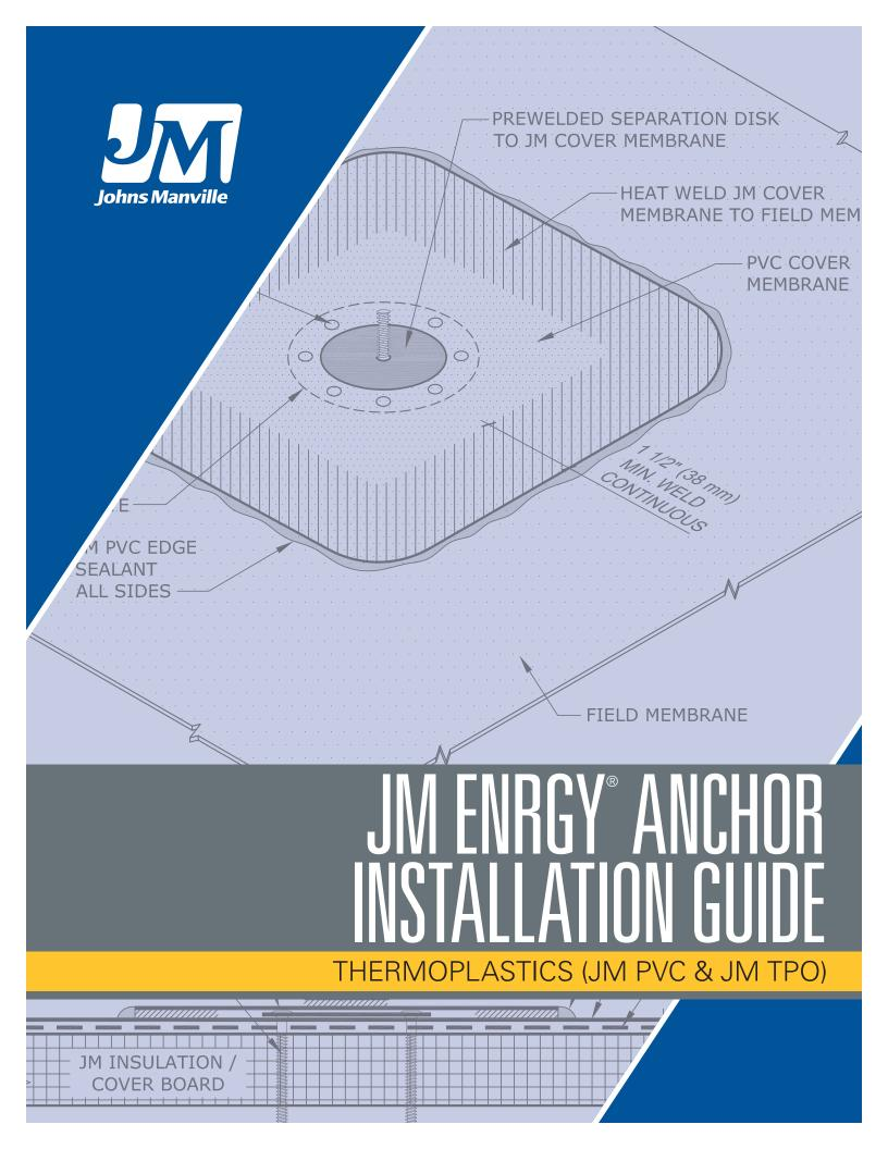
JM ENRGY<sup>™</sup> Anchor is a lightweight, roof-top integrated, photovoltaic (PV)-mounting solution consisting of a coated steel plate and stainless-steel stud and JM cover membrane.
