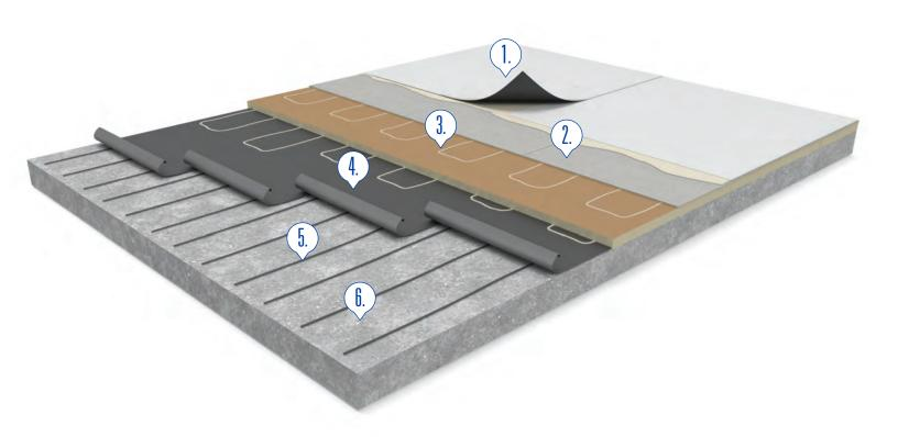
JM TPO – 80 mil, adhered in JM Membrane Bonding Adhesive (TPO & EPDM), JM LVOC Membrane Adhesive, JM TPO Water Base or JM All Season Sprayable Bonding Adhesive.
