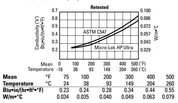
\*Apparent thermal conductivity values are determined by applying procedures dictated per ASTM C1045 on test data obtained using ASTM Test Method C335. All values are based on nominal manufacturing and testing parameters, are subject to normal variation, and are not guaranteed for specification purposes or otherwise.
