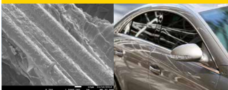
SEM picture indicating excellent matrix-glass bonding in PA6 system
