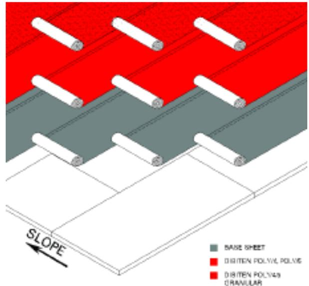
bleedout of compound shall be visible at the edge of all seams. All laps must be checked for good adhesion. Preparation of the 6" (152 mm) end lap requires scuffing away all loose granules. Heat and embed all remaining granules. Apply heat to the roll being seamed while making sure both have a good compound flow to adhere the two surfaces. End laps must be checked for proper adhesion.
