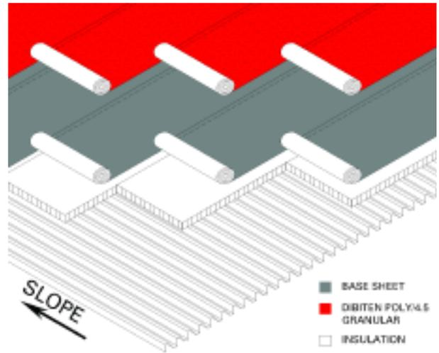
with 3" (76 mm) side and 4" (102 mm) end laps over the preceding sheets. Fasten the laps at 9" (229 mm) centers, and down the longitudinal center of each felt ply, place two rows of fasteners, with the rows spaced approximately 11" (279 mm) apart, and fasteners staggered on approximately 1/8" (457 mm) centers. Use fasteners appropriate to the insulation and deck.
