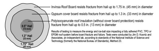
System performance in fully adhered JM Single Ply Roofing Systems
