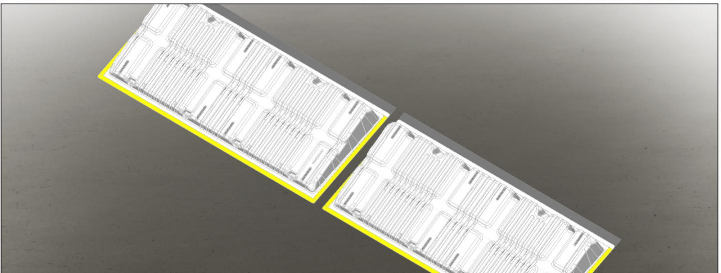
ENERGY Curbs in the field or north row of an array may overlap the neighboring south curb's TPO membrane depending on the inter-row spacing. Ensure the top surface of the ENERGY Curb's TPO membrane is properly cleaned before the peel-and-stick tape is overlapped. Tape application should be performed in temperatures above 50°F (10°C) to ensure best results.
