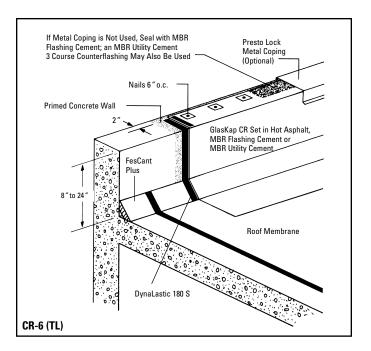
**Cold Adhesive Application:** When using cold adhesive, use a layer of MBR Flashing Cement  $\frac{1}{16}$ " (1.6 mm) thick, or a layer of MBR Utility Cement  $\frac{1}{6}$ " (3 mm) thick. Coat the parapet, the surface of the roofing membrane on the cant, and the roofing membrane on the field of the roof.
