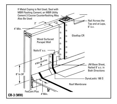
Hot Asphalt Application: Starting just above the point on the parapet where the base flashing will terminate, mop the parapet and the surface of the roofing membrane on and just below the cant. Holding the upper corners of the DynaLastic 180 S, position its lower horizontal edge on the cant and lay it into place over the cant strip and up the wall. The sheet should be "worked in" to ensure that it is firmly and uniformly bonded.
