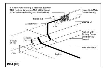
**Cold Adhesive Application:** When using cold adhesive, use a layer of MBR Flashing Cement  $\frac{1}{16}$  (2 mm) thick, or a layer of MBR Utility Cement  $\frac{1}{8}$  (3 mm) thick. Coat the parapet, the surface of the roofing membrane on the cant, and the roofing membrane on the field of the roof.
