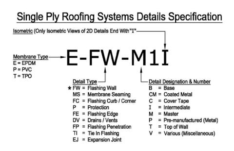
First is the designation for membrane type, followed by the designation for the area of installation, ending with the specific detail part (Base, Top of Wall, etc.) or material used in the detail (Coated Metal, Pre-Manufactured Metal, etc.). If there is an Isometric view of a two dimensional cut detail, the Isometric detail will end with an "I".
