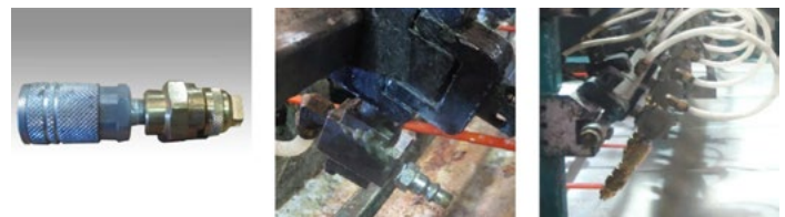
Water Spray Tip Assembly Existing Quick-Connect Fitting Installed Water Spray Nozzle
