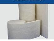
A lightweight insulation made from rotary-process fiberglass. Provides excellent thermal performance for commercial and residential applications operating at hot-face temperatures up to 1000° F. While Spin-Glas WH XG / Range-Glas XG is made with a formaldehyde-free binder, first exposures of the insulation to elevated temperature (≥ 450°F), will result in some formaldehyde emissions.
