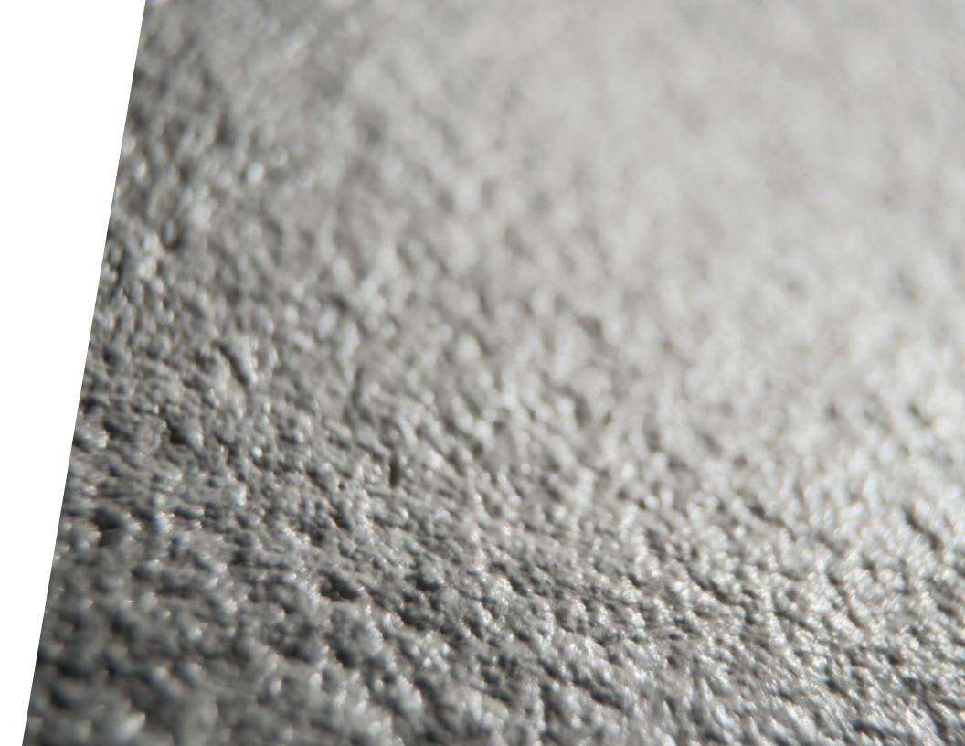
Made from inorganic glass fibers and bonded with a thermosetting resin, JM Insul-SHIELD® is a series of flexible, semi-rigid or rigid thermal and acoustical fiberglass boards for custom curtainwall applications. Where to use: acoustical ceilings, recording studios, curtainwall cavities, etc.
